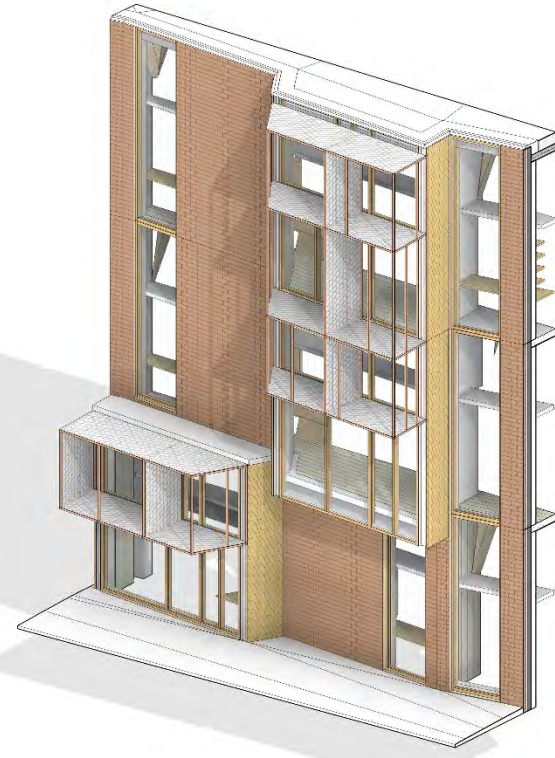
3D VIEW OF CLASSROOM FENESTRATION / SOLAR SHADING
